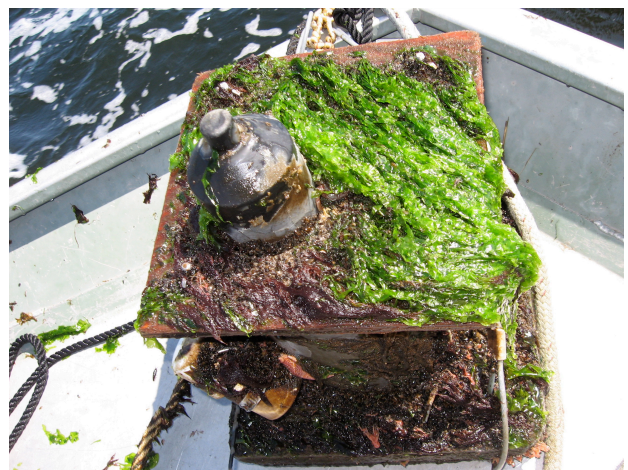
A receiver after a season of listening for fish. Every time a fish passes the receiver, its individual id, the date and the time are recorded.
